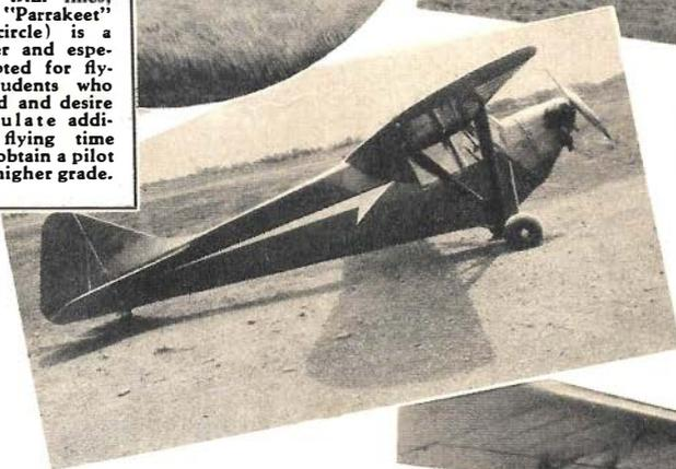
Increasing in popularity daily, the Taylorcraft (above) is one of the latest arrivals in the light plane field. The cabin features side-by-side seating and wheel-type controls in place of the conventional stick type. Prices of leading "flivver-planes" range from \$1,200 to \$1,800, with all models available on installment purchase plans featuring very liberal terms.
