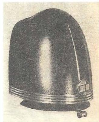
Entirely independent of the motor cooling system, the automobile heater shown above burns gasoline in a patented sealed metal chamber. The fuel is drawn in through a line tapped to the carburetor of the auto and, when mixed with air in a special venturi, burns as an extremely hot gas. The gas is ignited by turning on an electric heating element, which automatically shuts off in about 90 seconds.
