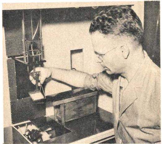
O. C. Hollstein, research engineer, adjusts the screen of a model fluoroscope exhibited at a radiologists' convention in Chicago. The model's floor is cut away to show x-ray tube.
