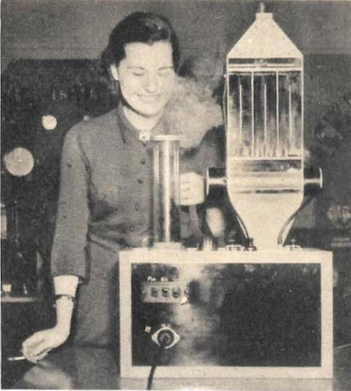
This electrostatic air cleaning machine removes dust, smoke and pollen from the air by ionizing particles and causing them to pass over grounded plates to which they cling. Young lady is shown testing the device with tobacco smoke.
