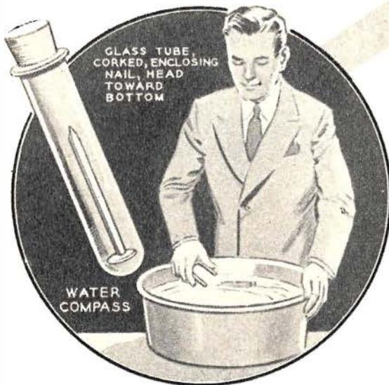
**WATER COMPASS**—Into a small vial or glass tube, place a small nail with the head toward the bottom of the vial. Cork it up and place it in a tumbler or pan of water. As the vial floats it is free to move in any direction. Then bring the magnet close to the vial but not touching it, and notice how it follows the magnet around the edge of the pan.
