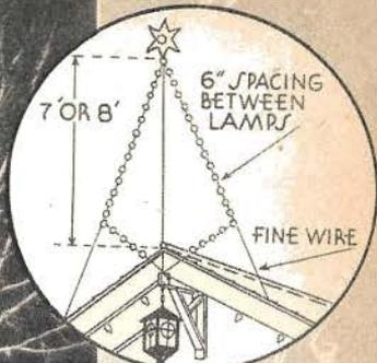
Housetop illuminated tree is formed with stringer lights. A 6- or 7-ft. vertical pole serves as support for the thin wires outlining tree.
