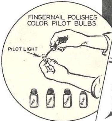
Ordinary fingernail polishes may be used for tinting colored pilot bulbs used to identify wave bands in all-wave radio receivers.
