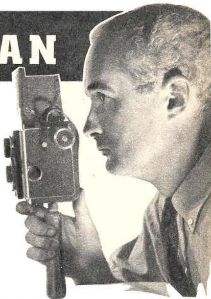
This useful handle-grip accessory will greatly simplify picture taking. It is made from an old soldering iron handle, fitted with a bolt of the correct size to fit into the tripod socket on camera.
