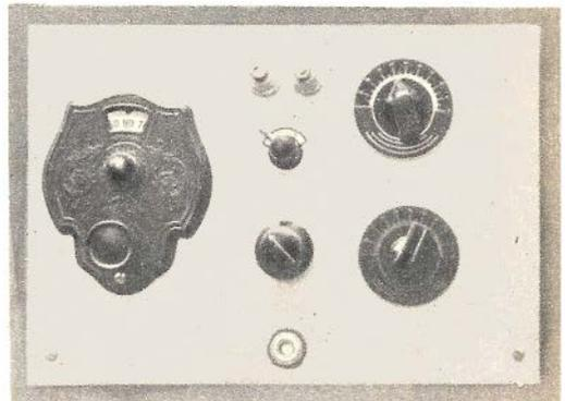
When the set is not in operation, be sure the changeover switch is either in the off position or on "transmitter." When the switch is in "receiver" position, the potentiometer and dropping resistor are connected across the "B" battery.
