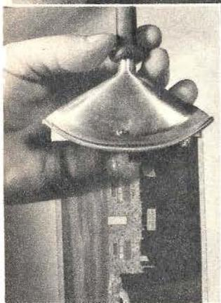
Films may be washed in  $\frac{1}{4}$  the usual time with this funnel kink. Flatten a 3-in. diameter aluminum funnel, punch a small hole in the side and insert a push-pin for supporting the cut film. To use, connect funnel to water hose.
