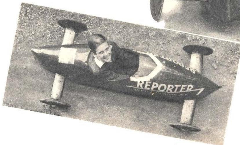
This view of Bob Ballard's soap box racer provides a clear conception of the streamlined design of the body, the faired axles and the road-hugging qualities imparted by the underslung design and wide-spaced wheels. Left—This top view shows the cigar-shaped body with tapering nose and tail. The driver's seat is just wide enough to admit pilot.
