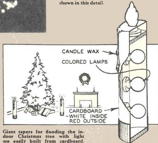
Giant tapers for flooding the indoor Christmas tree with light are easily built from cardboard. Back of candle forms floodlight.
