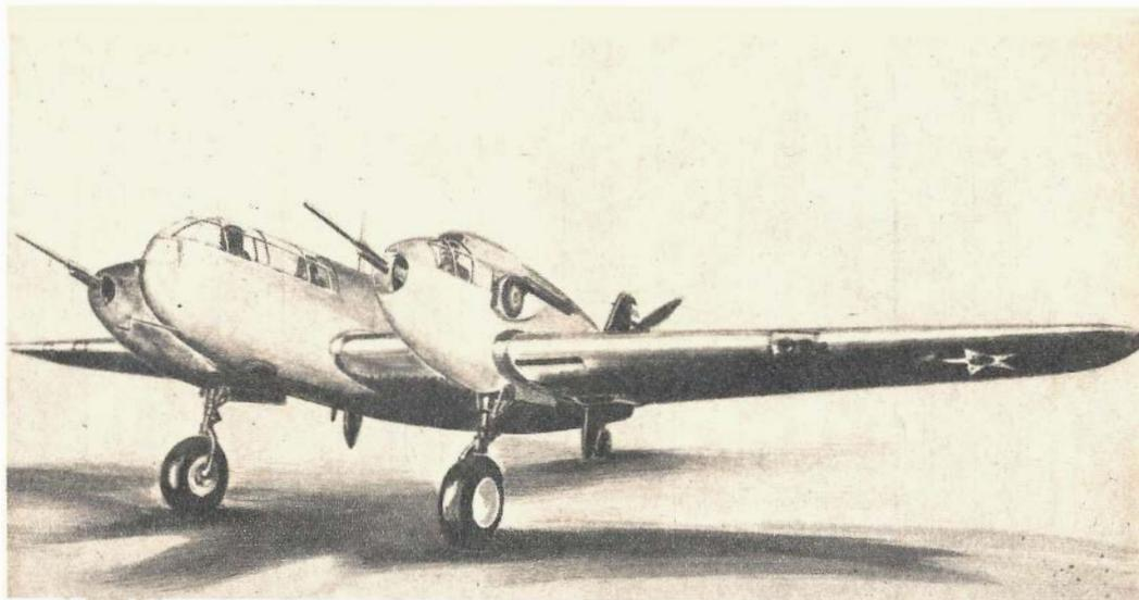
An artist's sketch of the XMF-1, a new type of pursuit plane developed for the U. S. Army Air Corps. Its twin pusher engines of 1,000 horsepower each are expected to drive it along at over 300 m.p.h. Full armament consists of six machine guns.
